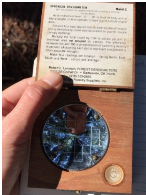
Figure 2: Densiometer Mirror, used to take canopy cover density measurements.
