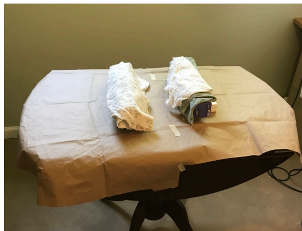
Temporary supports made using soft boxes and cotton rags. These will be used to support a specimen during cleaning and should be in place before the specimen is moved.
